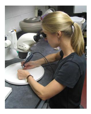
Figure 14. Sample cleaning under 10x magnification with a fine dental drill.
